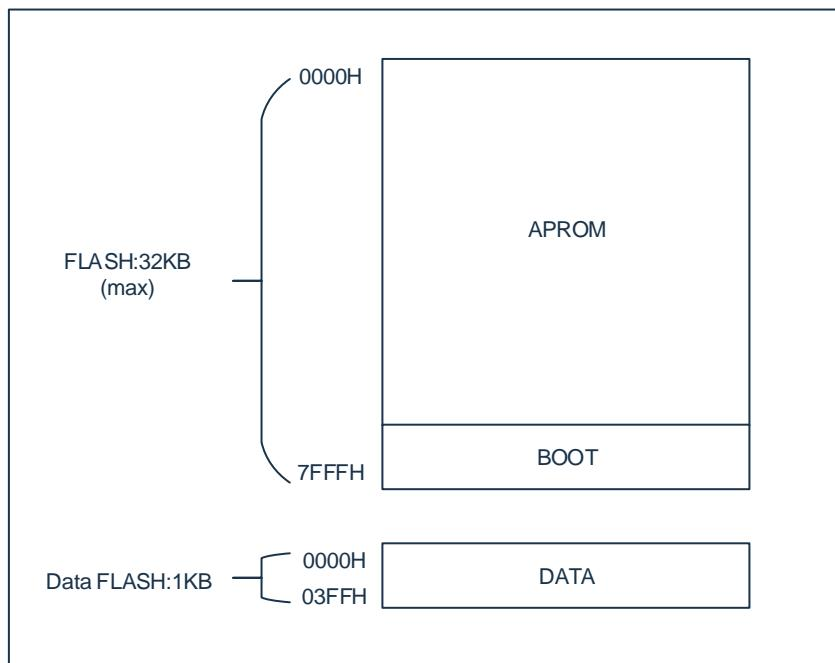
CMS80F751x can configure the size of BOOT, the configuration method is as follows:
