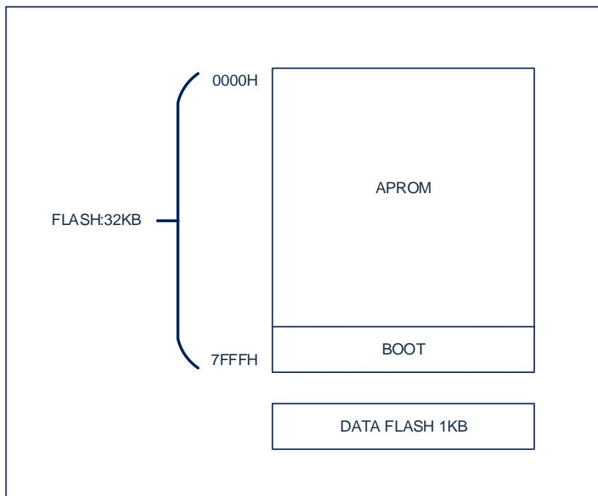
The size of BOOT can be configured, the configuration method is as follows:
