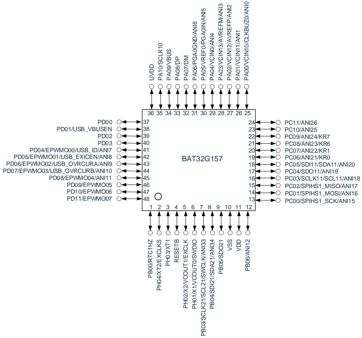
Note: The unmarked digital function support pins in the figure are configurable, see section 4.1 for details.
